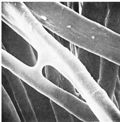
Fig. 8. Scanning electron micrograph of 11% polysiloxane-coated fibers. Magnification twice that of other figures.
